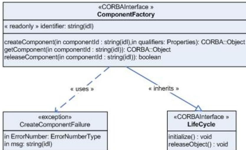
Figure 3-9: **ComponentFactory** Interface UML
